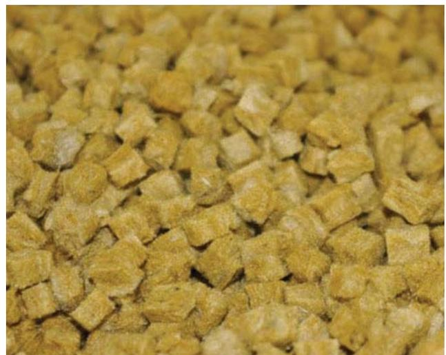
Figure 28. Horticultural rockwool used in potting media.
