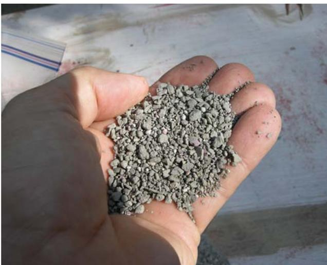
Figure 29. Calcined clay particles.
