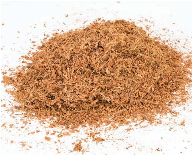
Figure 24. Shredded coconut fiber (coir).
